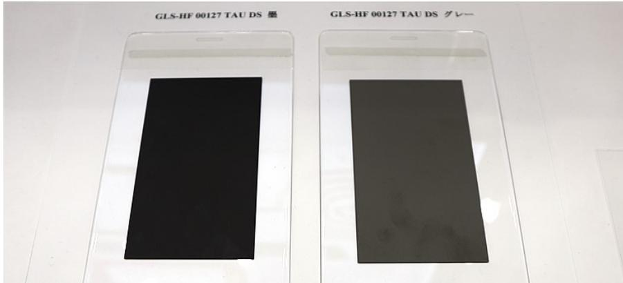
This is a printing example of MRX-HF 00127 TAU DS Black, Gray and Brown (substrate: PC) Because these can be printed in multiple layers, it is also possible to pursue both shielding function and designability by using MRX-HF 00127 TAU DS Brown, which has a high shielding effect.
